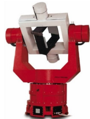
3-axial turntable with built-in temperature chamber for analysis of complex rotation movements
