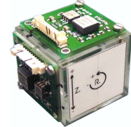
Inertial Measurement Unit for capturing complex movements in space
